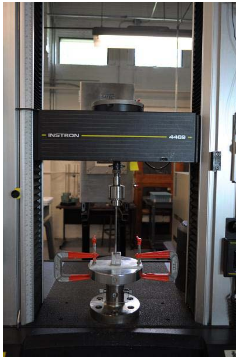
Figure 5.6. Tooth Setup for Fatigue Test in Instron 4469
